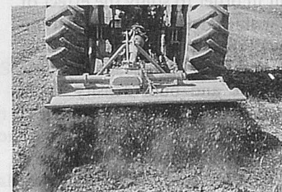
Fig. 5 Rotary tiller in operation (Shield up).
