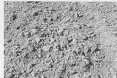
Fig. 16 Rotary tilled plot at speed-III and rear shield down.
