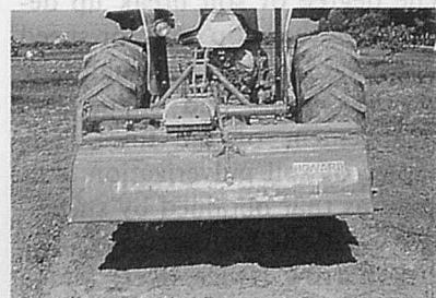
Fig. 1 Rear view of rotary tiller (Shield down).
