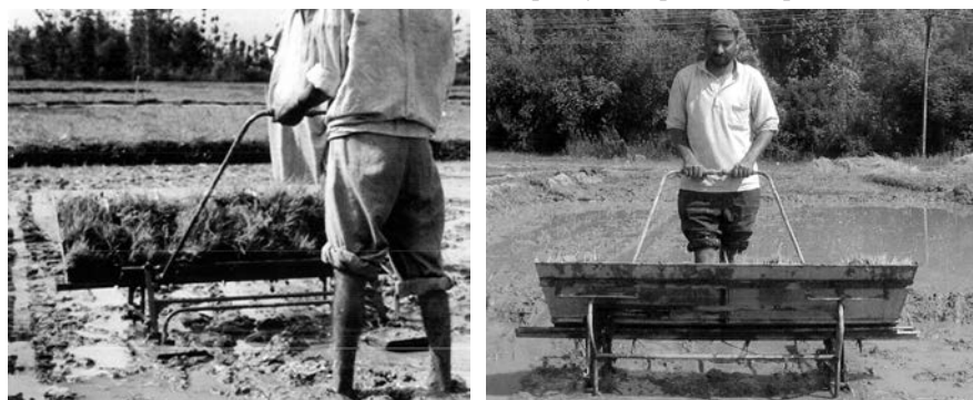
Fig. 2 Rear and front view of manual paddy transplanter in operation
