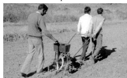
Fig. 3 Manual multi-crop planter in operation
