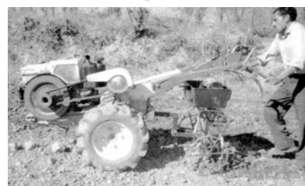
Fig. 4 Power tiller multi-crop planter in operation
