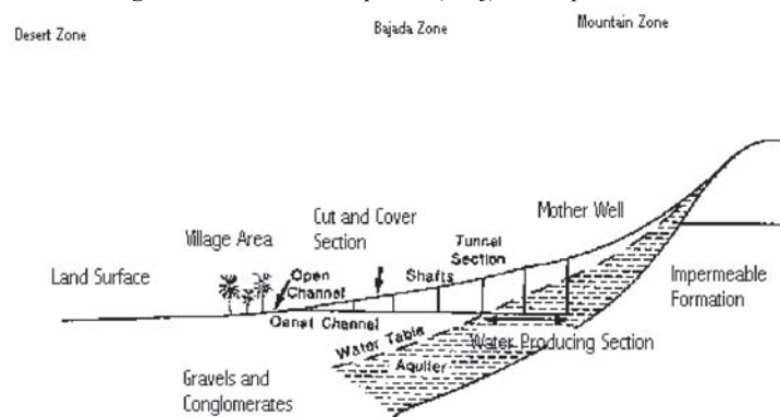
Fig. 3 Cross-section of qanat (falaj) in the piedmont zone
