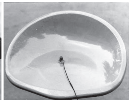
Fig. 3 Accelerometer placed on metallic seat of power tiller B
