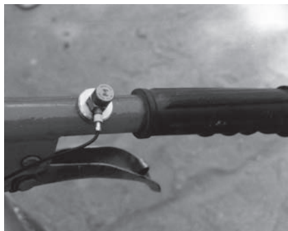
Fig. 2 Accelerometer on handle of power tiller A
