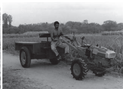
Fig. 2 View of the measurement of heart rate during the operation of power tiller A with trailer attachment on farm road
