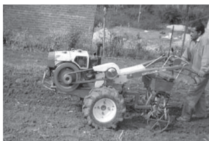
Fig. 2 Power tiller operated multicrop planter and manual planter in operation
